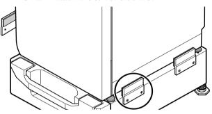
Be sure to press the adhesive parts of the brackets firmly to the appliance.
